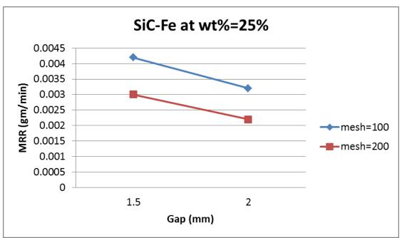
Figure (16) Relationship between gap size and metal removal rate at concentration 25% Si
