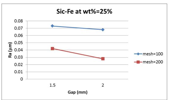
Figure (8) Relationship between gap size and surface roughness at 25% Si
