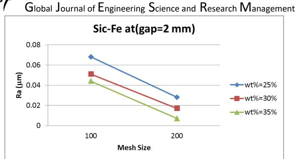
Figure (7) Relationship between mesh size and surface roughness at gap 2mm
