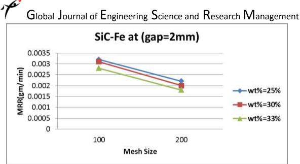
Figure (15) Relationship between mesh size and metal removal rate at gap 2mm
