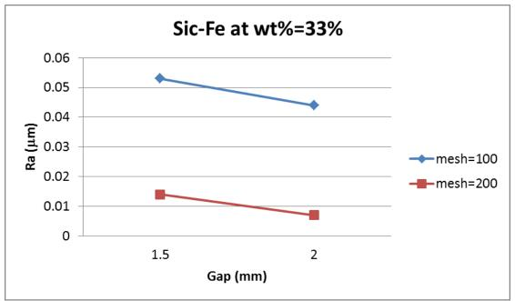
Figure (10) Relationship between gap size and surface roughness at concentration 33% Si
