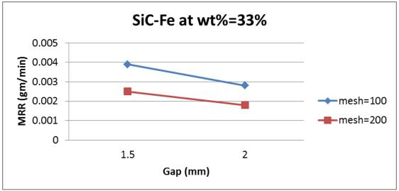
Figure (18) Relationship between gap size and metal removal rate at concentration 33% Si
