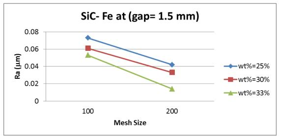
Figure (6) Relationship between mesh size and surface roughness at gap 1.5mm
