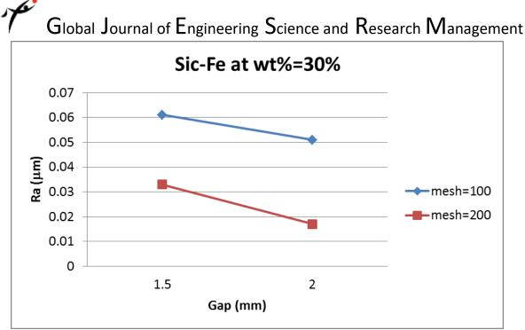
Figure (9) Relationship between gap size and surface roughness at 30%Si
