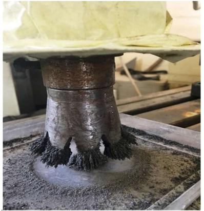
Figure (5) machine of MAF process
