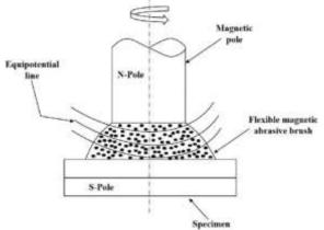
Figure (1) principle of MAF process [2]
