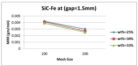
Figure (14) Relationship between mesh size and metal removal rate at gap 1.5mm
