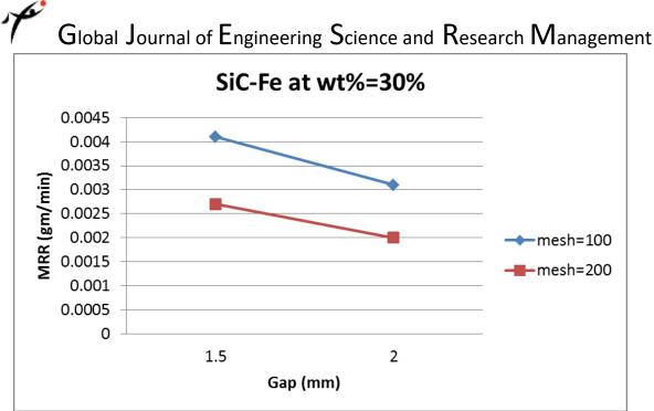
Figure (17) Relationship between gap size and metal removal rate at concentration 30% Si
