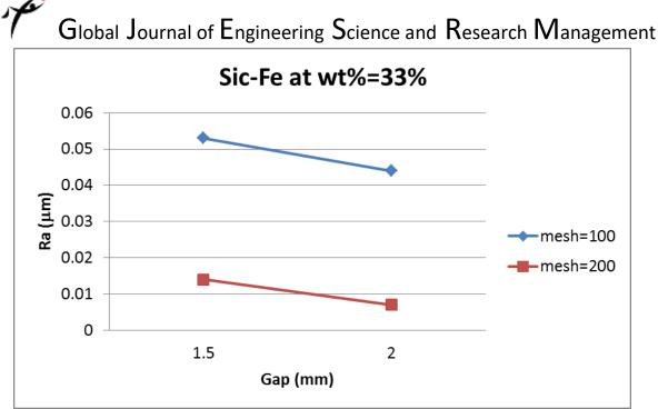
Figure (13) Relationship between mesh size and surface roughness at concentration 33% Si
