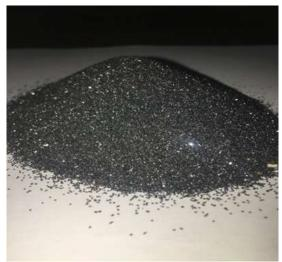
Figure (3) Abrasive of silicon carbide
